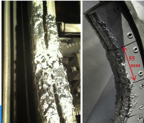
RE damage at T-10
