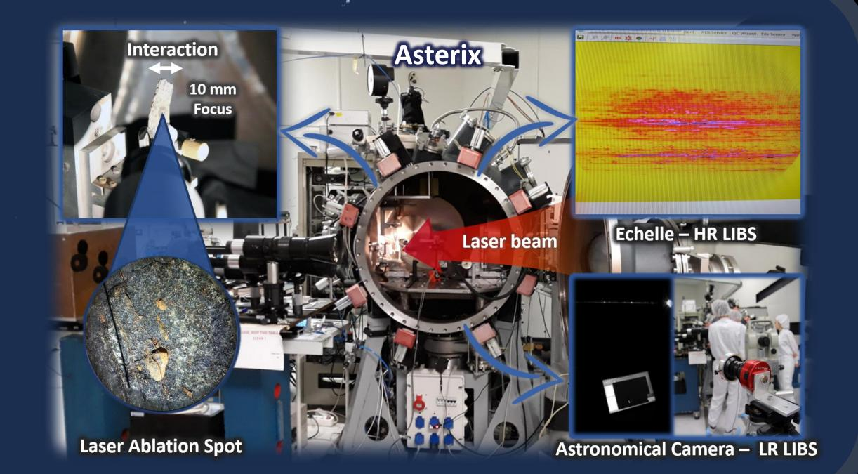
• High-resolution spectrum was measured using Echelle Spectrograph and the lowresolution spectrum was simultaneously obtained via an astronomical spectrograph.
