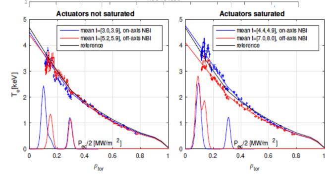
Controller works well as long as the gyrotrons are not at power limit (full/zero) In this case ~50% of the time Controller was optimized for this scenario!
