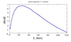
Simulated photon source energy: Maxwell-Boltzmann (MB) distribution with T in the range: 100 keV - 1 MeV with 100 keV step; 1 MeV - 50 MeV with 1 MeV step.
