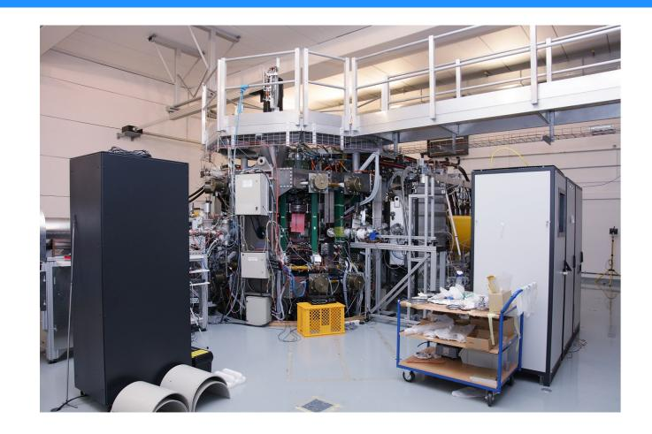
the tokamak COMPASS is compact size tokamak located in Prague G fields of research: H-mode physics, physics of plasma edge, plasma wall-interaction, physics of runaway electrons and disruptions etc.
