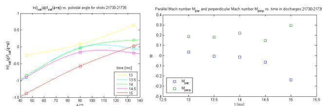
Figure 6: (a) Ratio of Ion saturation currents on Mach probe angle. ( $90^\circ$ -flow is perpendicular to the electrode surface); (b) Perpendicular  $M_{\perp}$  and parallel  $M_{\parallel}$  Mach numbers in time.
