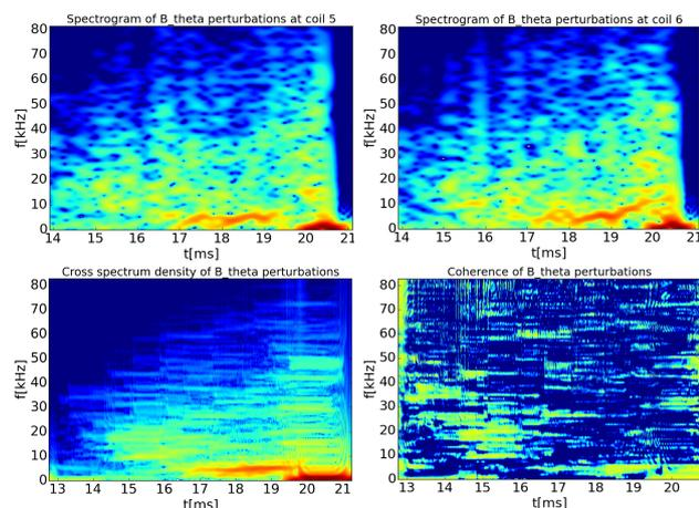
Figure 3: Spectrograms of perturbation of  $B_\theta$  measured at coils 5 and 6, their cross-spectrum time evolution  $S_{xy}$  and their spectral coherence. Discharge #10579.
