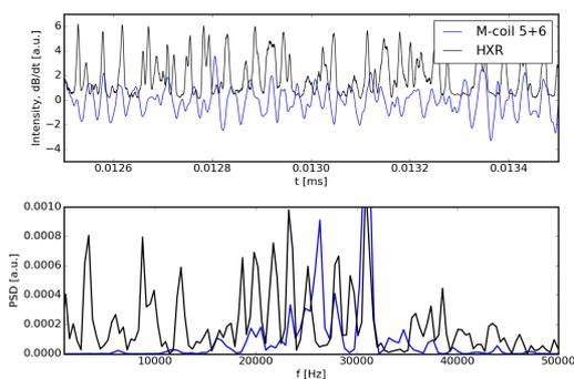
Figure 2: Convolved signal of neighbouring Mirnov coils compared to smoothed HXR signal in the time range where strong correlation is expected (top), power spectral density of these signals (bottom). Discharge #21501.
