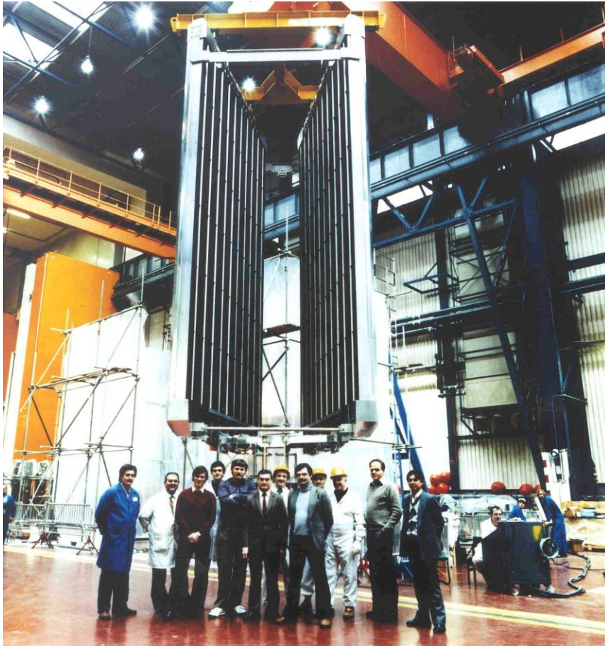
JET Neutral Injector cryopump.
