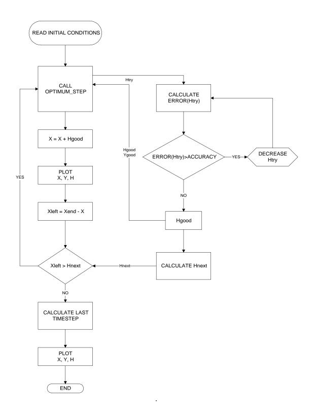
Figure 7: Flow chart for adaptive Runge-Kutta method.
