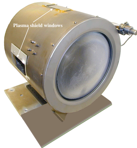
Fig. 1 – Photograph of the FMT-2 ion thruster indicating side and top plasma shield windows (bottom window not shown).
