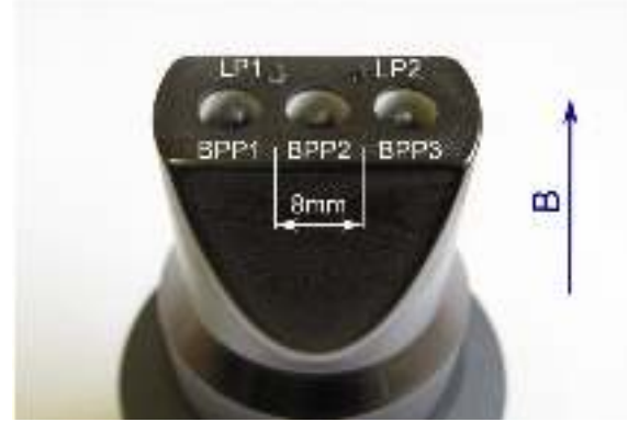
Figure 3.3: The probe head carrying three ball-pen and two Langmuir probes installed on COMPASS, from [23].
