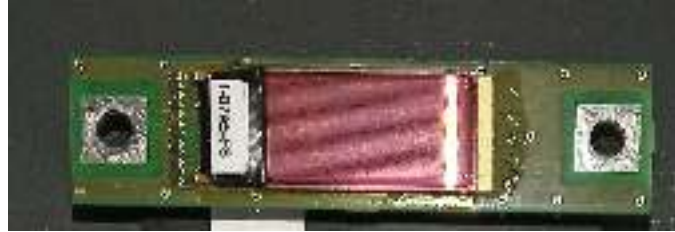
Figure 5.3: The 32-strip silicon detector is connected to PH32v8 readout chip.
