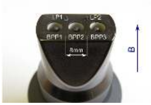
Figure 1. Probe head with three BPPs and two Langmuir probes. BPP3 is biased by a sweeping voltage at 50 kHz.
